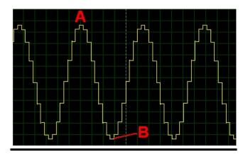
• 19 KHz Pilot Tone is synchronized with 38 KHz by Reset of 4015 Shift Registers
